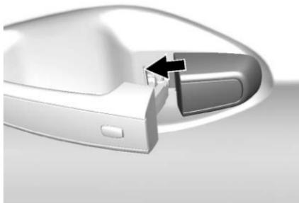
3. Move the cap forward and press to snap the cap in place.
