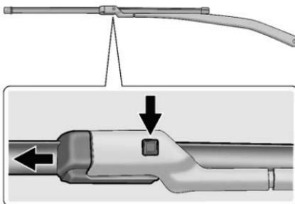
3. Press the button in the middle of the wiper arm connector, and pull the wiper blade away from the arm connector.
