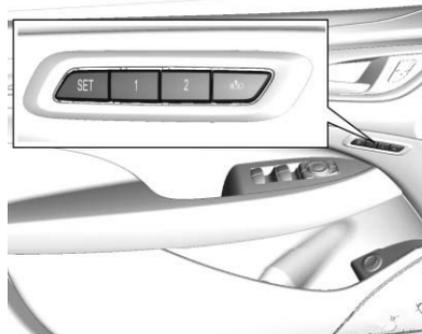
If equipped, the SET, 1, 2, and
