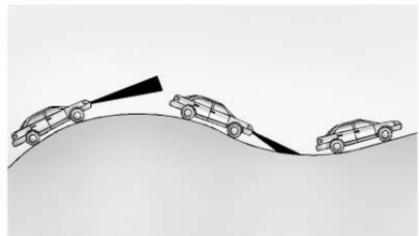
Do not use ACC when driving on steep hills or when towing a trailer. ACC will not detect a vehicle in the
