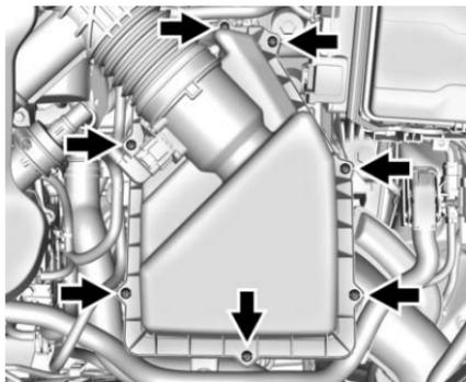
1. Remove the seven screws and lift the cover out of the assembly.
