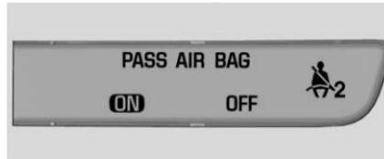
The words ON and OFF will be visible during the system check. When the system check is complete, either the word ON or OFF will be visible. See *Passenger Airbag Status Indicator* ⇨ 112.
