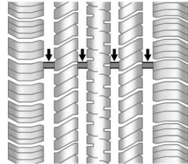
Treadwear indicators are one way to tell when it is time for new tires. Treadwear indicators appear when the tires have only 1.6 mm (1/16 in) or less of tread remaining. See *Tire Inspection* ⇨ 266 and *Tire Rotation* ⇨ 266.
