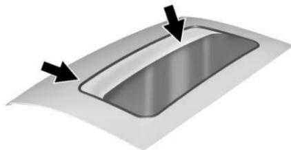
Dirt and debris may collect on the sunroof seal or in the track. This could cause issues with sunroof operation and noise. It could also plug the water drainage system. Periodically open the sunroof and remove any obstacles or loose debris. Wipe the sunroof seal and roof sealing area using a clean cloth, mild soap, and water. Do not remove grease from the sunroof.
