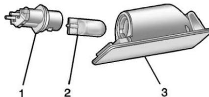
2. Turn the bulb socket (1) counterclockwise to remove it from the lamp assembly (3).
