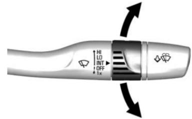
**INT** : Use for intermittent wipes. To adjust wipe frequency, turn the band up for more frequent wipes or down for less frequent wipes.
