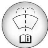
Open the cap with the washer symbol on it. Add washer fluid until the tank is full. See *Engine Compartment Overview* ⇨ 229 for reservoir location.
