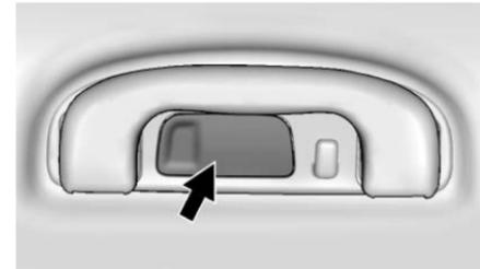
The rear reading lamps are over the rear passenger doors.
