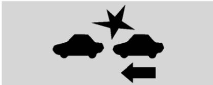
When your vehicle approaches another vehicle too rapidly, the red collision alert symbol on the HUD will flash on the windshield. Either eight beeps will sound from the front, or both sides of the Safety Alert Seat will pulse five times. When this Collision Alert occurs, the brake system may prepare for driver braking to occur more rapidly which can cause a brief, mild deceleration. Continue to apply the brake pedal as needed. Cruise control may be disengaged when the Collision Alert occurs.
