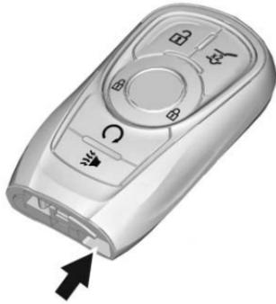
2. Insert a flat tool into the bottom of the transmitter and separate the transmitter into two halves.
