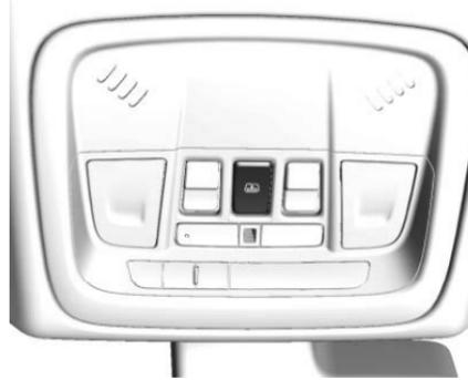
If equipped, the rear window sunshade button is on the overhead console. To open the sunshade, press and release. The sunshade will fully extend. To close the sunshade, press and release the switch again. The sunshade will fully close.
