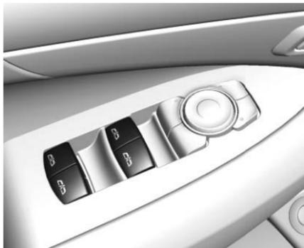
Windows with an express-up or down feature allow the front windows to be lowered or raised without holding the switch. Rear windows only have express-down. Pull a window switch up or press it down all the way, release it, and the window goes down or up automatically. Stop the window by pressing or pulling the switch.
