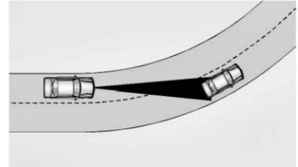
ACC may detect a vehicle that is not in your lane and apply the brakes.
