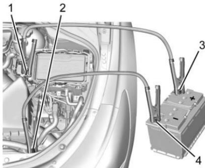
1. Discharged Remote Battery Positive Terminal
