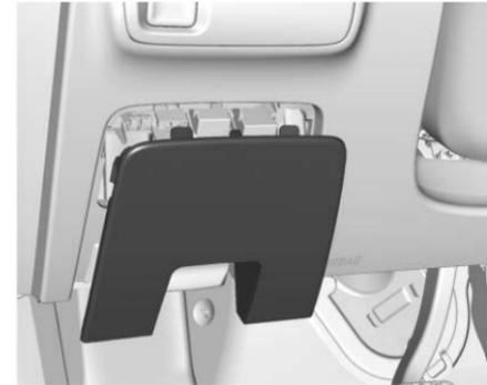
The instrument panel fuse block is in the instrument panel, on the driver side of the vehicle. To operate the fuses, open the fuse panel by pulling down at the top.
