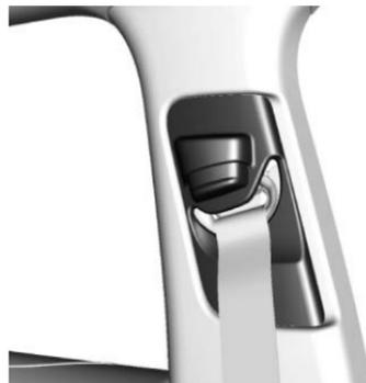
Press the release button and move the height adjuster to the desired position. The adjuster can be moved up by pushing the slide/trim up. After the adjuster is set to the desired position, try to move it down without pushing the release button to make sure it has locked into position.
