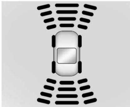
The instrument cluster may have a Parking Assist display with bars that show “distance to object” and object location information for RPA, and on some vehicles, FPA. As the object gets closer, more bars light up and the bars change color from yellow to amber to red.
