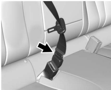
3. Reconnect the rear safety belt mini-latch to the mini-buckle. Do not let it twist.
