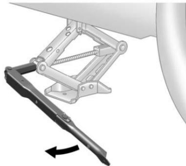
10. Raise the vehicle by turning the jack handle clockwise. Raise the vehicle far enough off the ground so there is enough room for the road tire to clear the ground.
