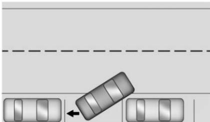
APA will instruct the vehicle to stop once a large enough space is found. Follow the instructions in the DIC. When instructed to drive in reverse, shift to R (Reverse) to engage automatic steering. The steering
