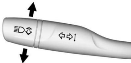
Move the lever all the way up or down to signal a turn.
