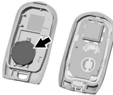
5. Insert the new battery, positive side facing up. Push the battery down until it is held in place. Replace with a CR2032 or equivalent battery.
