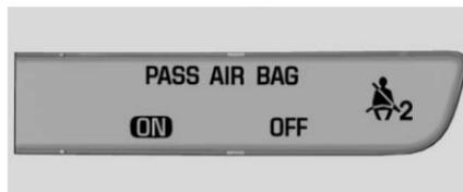
When the vehicle is started, the passenger airbag status indicator will light ON and OFF for several seconds as a system check. Then, after several more seconds, the status indicator will light either ON or OFF to let you know the status of the front outboard passenger frontal airbag and knee airbag.
