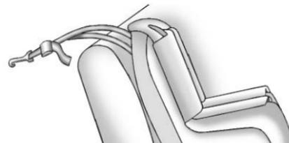
If the position you are using does not have a headrest or head restraint, or the headrest or head restraint has been removed, and you are using a dual tether, route the tether over the seatback.
