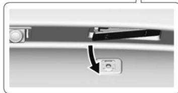
1. Push the lamp assembly toward the center of the vehicle, then move the lamp downward, and remove it from the vehicle body.
