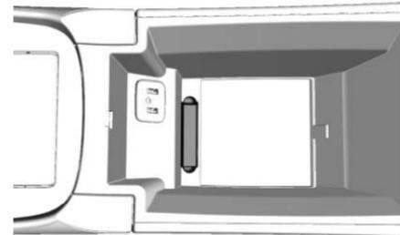
5. Place the new transmitter into the transmitter pocket inside the armrest storage area.
