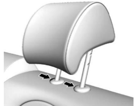
2. Press both buttons on the head restraint posts at the same time, and pull up on the head restraint.
