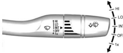
With the ignition in ACC/ACCESSORY or ON/RUN/START, move the windshield wiper lever to select the wiper speed.
