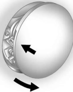
To open the fuel door, push and release the rearward center edge of the door.
