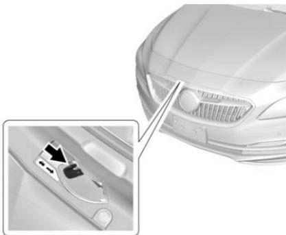
2. Go to the front of the vehicle and push the secondary hood release handle toward the driver side of the vehicle.
