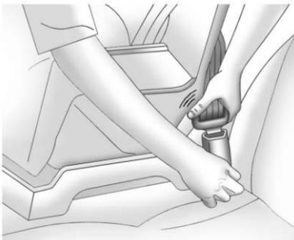
4. Push the latch plate into the buckle until it clicks. Position the release button on the buckle, away from the child restraint system, so that the safety belt could be quickly unbuckled if necessary.
