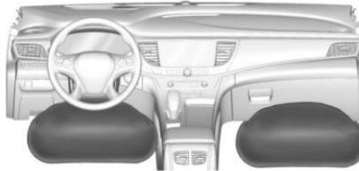
The driver knee airbag is below the steering column. The front outboard passenger knee airbag is below the glove box.
