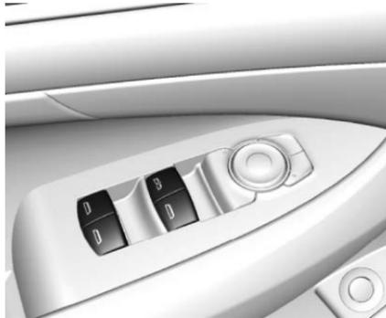
The switches work when the ignition is in ON/RUN or ACC/ACCESSORY, or in Retained Accessory Power (RAP). See *Retained Accessory Power (RAP)* ⇨ 177.
