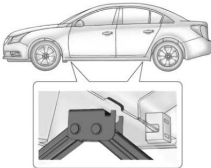
9. Position the jack lift head at the jack location nearest the flat tire. The location is indicated by a notch in the vertical bottom edge of the body side sheet metal.
