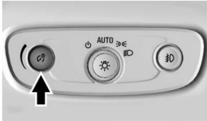
The brightness of the instrument cluster display, infotainment display and controls, steering wheel controls, and all other illuminated controls, as well as feature status indicators can be adjusted.
