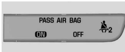
The passenger sensing system turns off the front outboard passenger frontal airbag and knee airbag under certain conditions. No other airbag is affected by the passenger sensing system. See *Passenger Sensing System* ⇨ 71.
