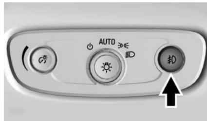
The fog lamps button is on the instrument panel to left of the steering wheel.
