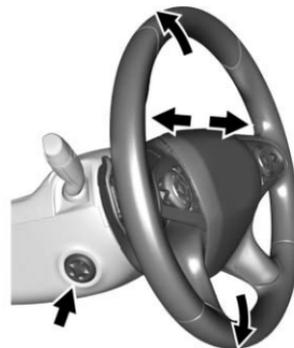
To adjust the steering wheel, if equipped:
