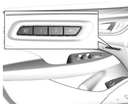
If equipped, the SET, 1, 2, and
