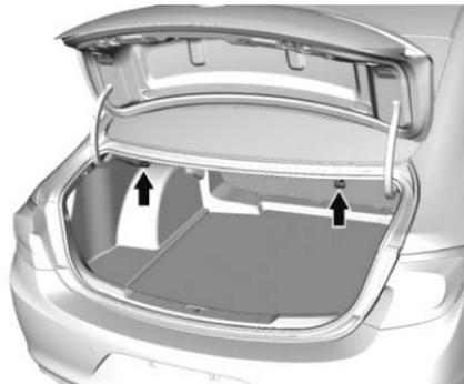
4. Pull the release cable in the trunk to fold the rear seatback down.
