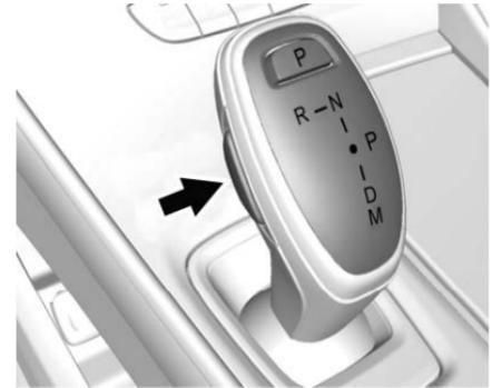
This vehicle is equipped with an electronic transmission. The shift lever unlock button is designed to prevent inadvertent shifting out of P (Park) unless the ignition is in ON/RUN, the brake pedal is applied, and the shift lever unlock button is pressed.
