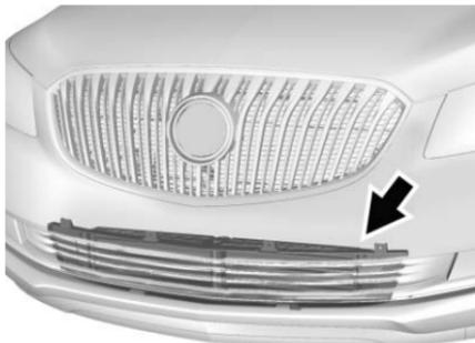
The vehicle may have a shutter system designed to help increase fuel economy. Keep the shutter system clean for proper operation.
